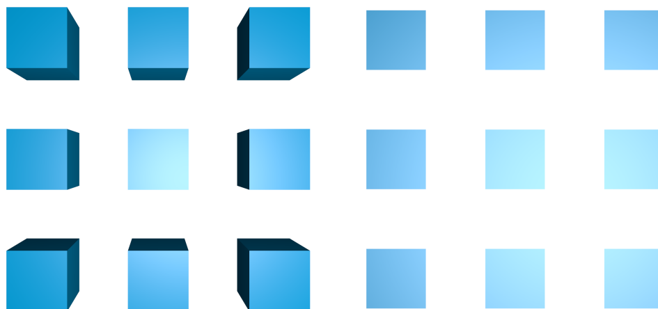
Figure 6.2: 9 cubes rendered using perspective projection on the left and in orthographic projection on the right.
